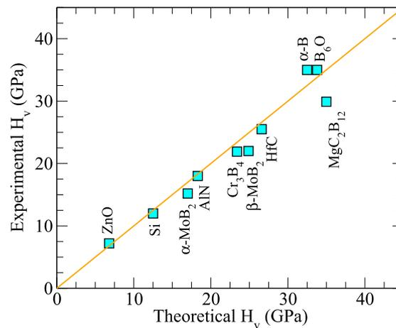
**Fig. 2.** A comparison of the available experimental Vickers hardness ( $H_v$ ) data with the theoretical values obtained using the recommended model in Section 5.1 for several materials listed in Table 2.
