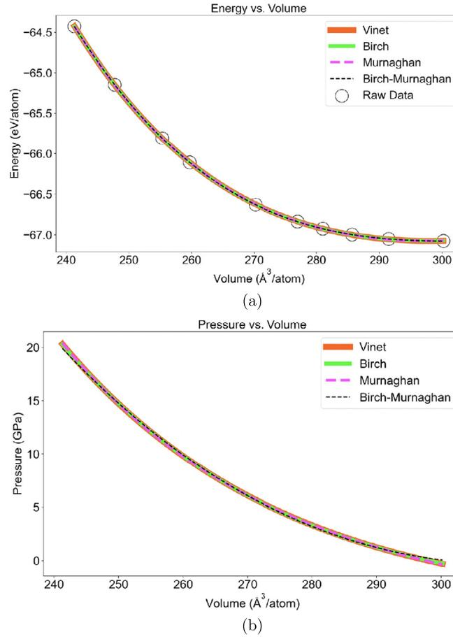
**Fig. 3.** The fitted equation of state (EOS) plots for (a) Energy vs. Volume and (b) Pressure vs. Volume data obtained by differentiating the energy with a central difference scheme using different EOS models. Here, the material under investigation is  $T_d$ -MoTe<sub>2</sub> for which ‘Energy vs. Volume’ data was computed using the VASP code (numerical details are given in Ref. [105]).
